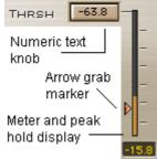
Each Band has its own meter showing the input energy in that band. Under the meter is a peak hold numeric indicator. When you want to set your nominal thresholds you can use the peak as reference and then continue to set them with the master threshold control.
